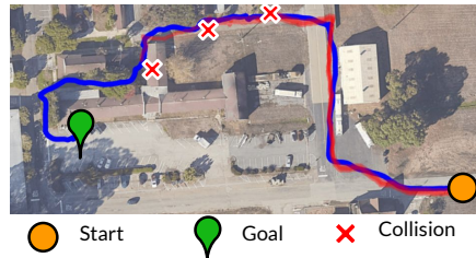
Figure 6: LM-Nav with a GPS-only controller fails to execute a plan due to its inability to reason about traversability through obstacles.
