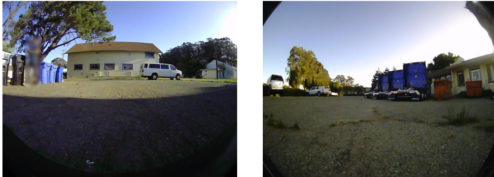
Figure 8: An example of failure to pick the correct image by maximum likelihood planning. Both images were selected for a prompt A photo of a blue dumpster . The left one was selected as a part of the LM-Nav’s graph search and the right was selected by maximum likelihood planning. In the latter case, the selected image contains a blue semi-truck and an orange trailer, but no blue dumpsters. This might be an example of an issue with the variable binding. The left image was edited to maintain anonymity.
