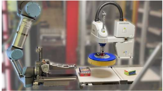
Fig. 4: Orientation EoAT and Hand-off: A SCARA robot with a foam disk is used to orientate items before they are conveyed into the robot EoAT.
