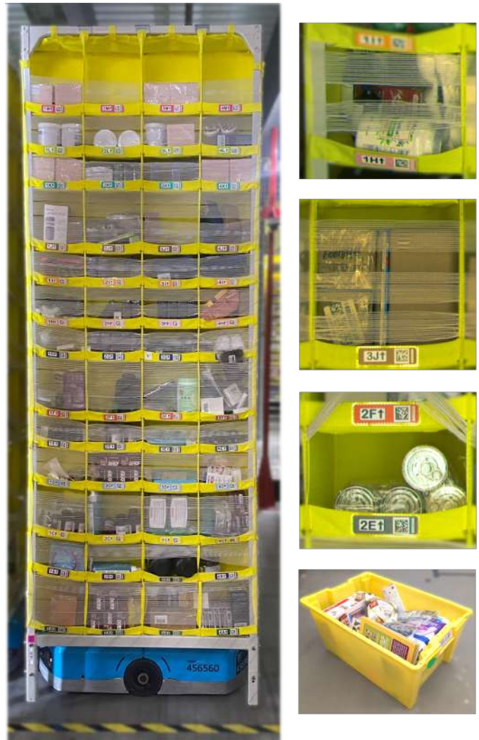
Fig. 1: Storage Pod: Items are stored densely and heterogeneously within each bin on this pod face. Elastic bands are used to prevent objects from falling out as pods are moved throughout the building by mobile robots. Bins are continuously picked from and stowed into during operations. Items arrive at stow stations in plastic totes, bottom right.
