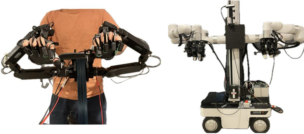
Figure 2: **Mobile bimanual teleoperation system** Left: An operator strapped into BiDex. Right: Our bimanual robot setup including two xArm robot arms, two LEAP Hands [1] and three cameras on an AgileX base.
