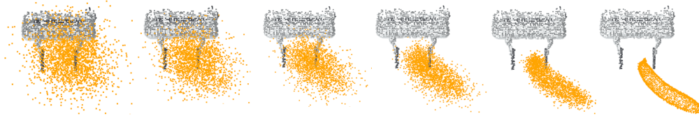
Figure 3. Trajectory of the pick generation process (“grasp the banana by the crown”). Unlike the place generation, our pick generation is conditioned on the canonicalized gripper point cloud. The generated point cloud at each timestep is colored in orange.
