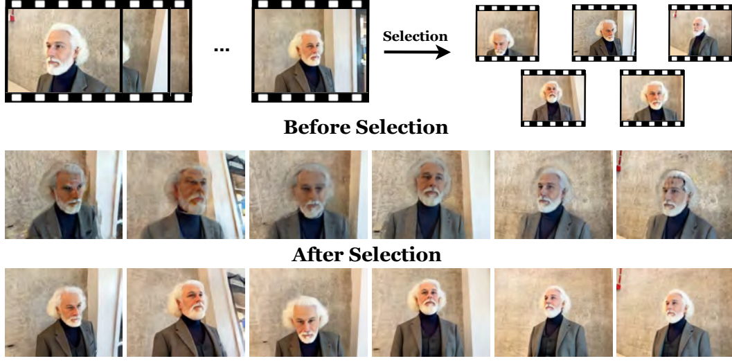
Figure 7: To mitigate the inconsistency issue, EditCast3D first employs CF-3DGS (Fu et al., 2024), a pose-free 3D Gaussian Splatting reconstruction method, to obtain an initial reconstruction of the scene. Training views with higher PSNR are then identified as more consistent views and selected. These selected views are subsequently passed to InstantSplat (Fan et al., 2024) to perform the final feedforward reconstruction for improved consistency and quality.
