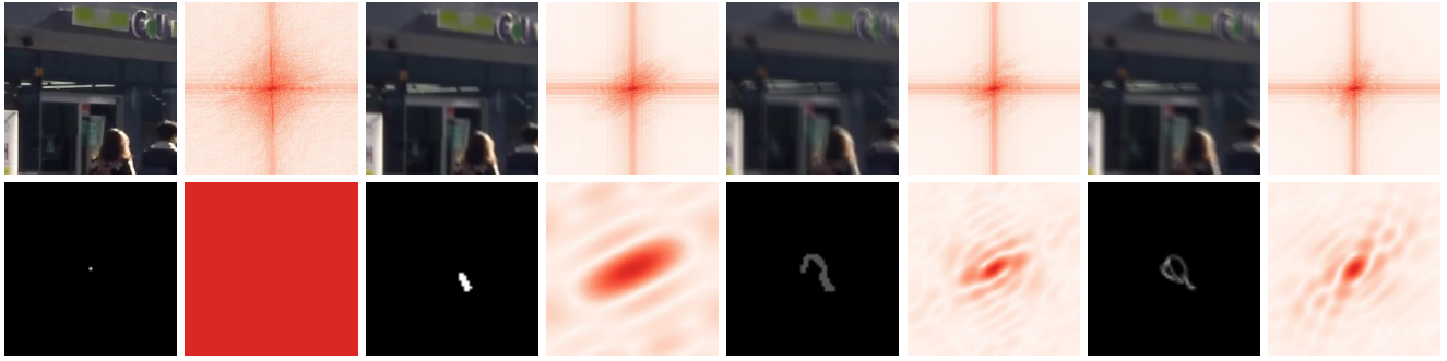
Figure 3: The visualization of various generated kernels and their impact on the sharpness of images within both the spatial and frequency domains. Specifically, the first row of the visualization pertains to the degraded image, while the second row illustrates the generated kernel. Furthermore, the odd columns represent the spatial domain, while the even columns depict the frequency domain.
