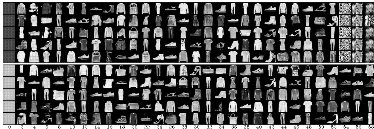
Figure 16: The generated images from the noise-free GAN and the noised GAN. Upper : Noise-free GAN. Lower : Noised GAN. The noise-free GAN collapses at the 54th epoch, whereas the noised GAN consistently produces high-quality images.
