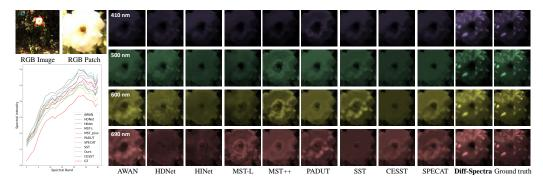
Figure 4: Visual comparisons on a randomly selected scene from the validation set of the ARAD-1K dataset with 4 spectral channels. The spectral curves (bottom-left) correspond to the selected blue Box of the RGB image. Please zoom in for a better comparison.
