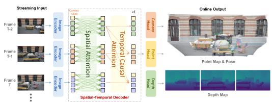
Figure 3: **Framework of StreamVGGT.** Our model consists of three main components: an image encoder, a spatio-temporal decoder, and multi-task prediction heads. During training, we utilize full-sequence inputs to provide the model with complete contextual information. To enforce temporal causality, we apply causal attention so the model can only attend to past frames at any given time step. This design encourages realistic temporal modeling suitable for streaming inference.
