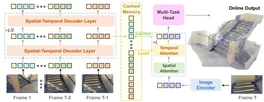
Figure 4: **Efficient inference of our model.** During streaming inference, we cache the historical keys and values as implicit memory to store information from past frames. This memory allows the model to efficiently reuse previously computed representations, avoiding redundant computation and enabling consistent contextual understanding across time. Our model then processes input incrementally and achieves performance that is comparable to full-sequence inference.
