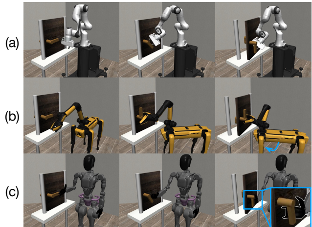
Fig. 4: Rollouts from policies trained using 3D object flow as a reward. Different embodiments such as the (a) Panda, (b) Spot, or (c) GR1 use different strategies to open the door. The Spot is able move its base for better reachability while the GR1 uses the area between its fingers and palm to pull for better stability.
