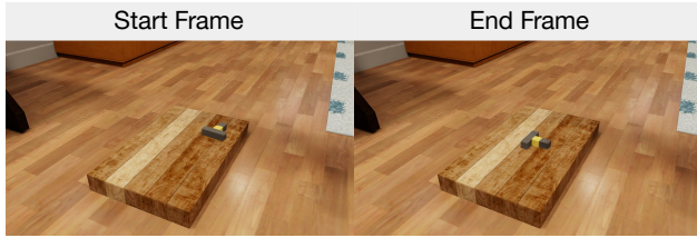
Fig. 7: Example Push-T image prompt. To generate sufficiently accurate motions for the Push-T task, the visual component of the prompt includes both a start and end frame.
