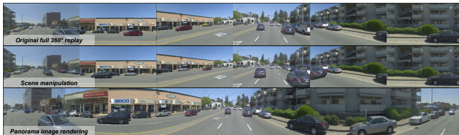
Fig. 8: Realistic and controllable multi-camera simulation on PandaSet. G3R reconstructs a manipulable 3D scene representation.
