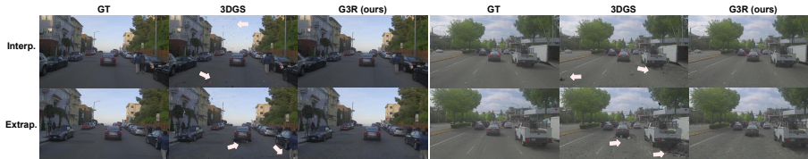
Fig. 6: Robustness of G3R vs. 3DGS. 3DGS is sharper on interpolation views ( Interp. ), but has artifacts on extrapolation views ( Extrap. ).
