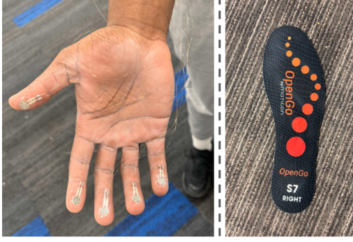
Figure 3. Our hand contact sensors cause only minor changes to the appearance of the hands and are nearly imperceptible. The commercially available foot sensor is inside the shoes, which is completely invisible.
