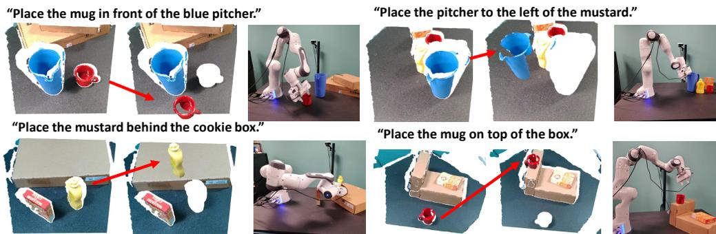
**Figure 1:** Planning to achieve different predicate relationships in the real world, given only segmented point clouds of the scene. The planner computes final placement positions and associated kinematic poses, which lets the robot generate a motion plan to place these objects at different locations in the real world.
