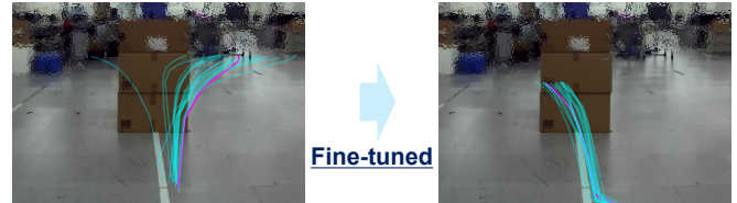
Fig. 2. Less divergent trajectory generation after fine-tuning. Based on a shared start-goal and an observation point, we visualize N = 20 trajectories sampled from each model: Left : the zero-shot NoMaD (before being fine-tuned); Right : the fine-tuned model. Fine-tuning yields markedly lower diversity, with narrower spatial spread and reduced heading variance, indicating a collapse of pretrained priors.
