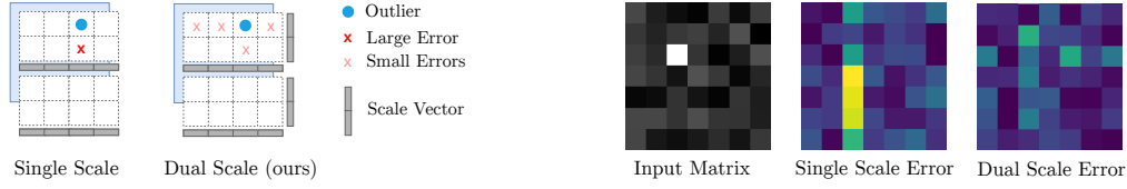
Figure 1: If we have scales along both dimensions of a matrix that is to be quantized, we can trade off the impact of outliers between rows and columns, which is impossible in single-scale quantization. Left: Conceptual illustration of error distributions with single or dual-scaling. Right: Example on small matrix.
