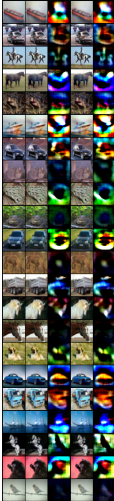
Figure 8: Illustrative examples of attack performance. Each column (from left to right) represents: the original image; the image under our attack; the adversarial perturbation associated with our attack; the image under PGD; the adversarial perturbation associated with PGD. The adversarial perturbations have been multiplied by 25 for visual clarity.
