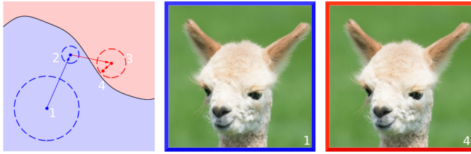
Figure 1: An illustrative evasion attack for a binary classifier, where knowledge of the certifications (circles) allows an iterative attack to better optimise their attack .
