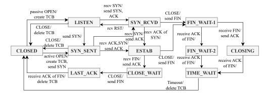
Figure 5: A manually extracted ground-truth PSM of TCP protocol in RFC2PSM.
