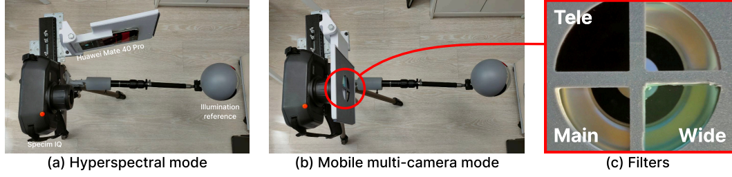
Figure 4: Capture setup for the Doomer dataset. (a) Smartphone holder rotated to allow hyperspectral capture via Specim IQ. (b) Smartphone repositioned for simultaneous multi-camera RGB capture. (c) External spectral filters mounted on Tele and Wide cameras to induce spectral diversity.
