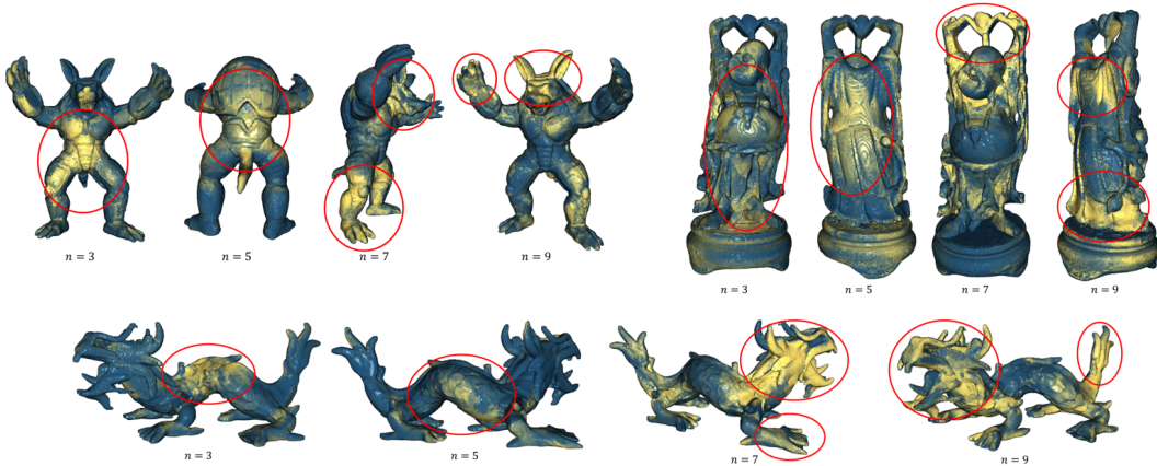
Figure 7: Shape compression result of our model by using the data from Stanford University (2023). n means the dimensionality of features, and they are performed individually. The greater the magnitude of the gradient, the more yellow it is.
