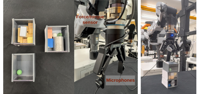
Fig. 1. Long-horizon stacking task by multimodal large language models. Left: Three containers to be stacked with various contents. Middle: Multimodal sensing setup for object hidden properties. Right: The NEXTAGE robot performing box stacking guided by an LLM.
