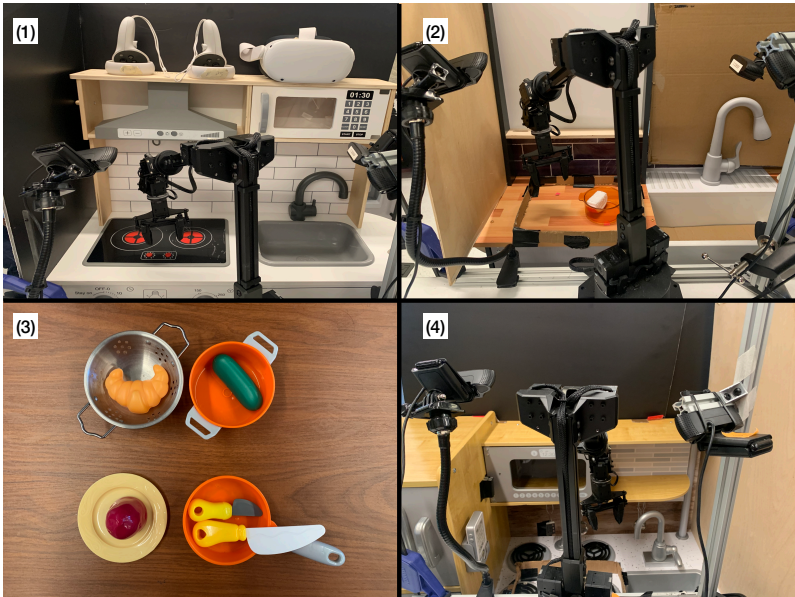
Figure 7: Setup Overview: Following Ebert et al. (2021), we use a toykitchen setup described in that prior work for our experiments. This utilizes a 6-DoF WidowX 250 robot. (1): Held-out toykitchen used for experiments in Scenario 3 (denoted “toykitchen 6”), (2): Re-targeting toykitchen used for experiments in Scenario 2 (denoted “toykitchen 2”), (3): target objects used in the experiments of scenario 3., (4): the held-out kitchen setup used for door opening (“toykitchen 1”).
