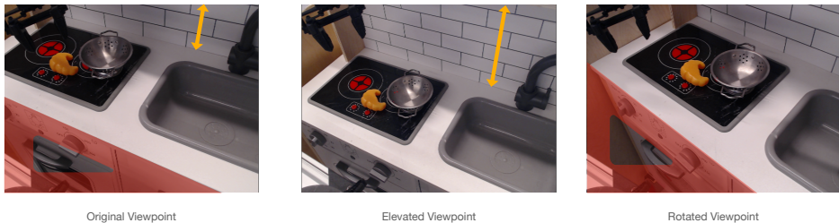
Figure 14: Sample observations from different camera viewpoints, only used during fine-tuning. Left: the original camera viewpoint found in Figure 13. Middle: an elevated camera viewpoint where the robot and camera has been raised 7 cm. Right: a rotated camera viewpoint where the kitchen has been slightly translated and rotated 15 degrees counterclockwise relative to the camera and robot.
