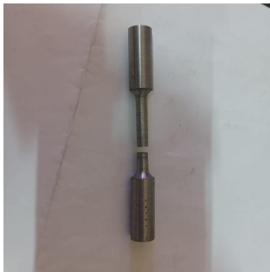
Fig: - Dogbone specimen undergone fracture after tensile testing
