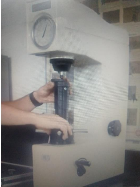
Fig: - Rotate the wheel to ensure that the diamond cone indenter comes in proper contact with the specimen.
