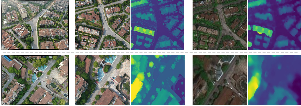
Figure 11: Visualization of reference maps with different quality levels. The left shows the query image, the middle displays the RGB-Depth pair rendered from the high-quality map, and the right shows the RGB-Depth pair from the low-quality map. Although the maps are geo-aligned, the low-quality version exhibits degraded appearance and reduced geometric accuracy.
