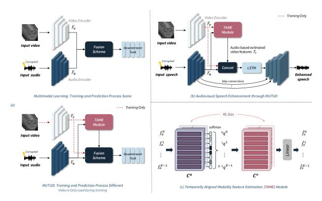
Figure 1: (a) The left panel shows a comparison between conventional audiovisual speech processing and MUTUD. TAME module enables audiovisual learning without doing video processing during prediction. (b) The upper half in the right panel illustrates MUTUD for an AVSE model. After training the video encoder is discarded. (c) The bottom half in the right panel shows the estimation of video representations using TAME. The illustration is for t=0 in Eq 5.
