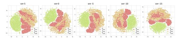
Figure 5: TSNE visualization of the estimated video features  $\hat{F}_v$ , the actual video features  $F_v$ , and the audio features  $F_a$  for SNRs ranging from 5dB to -15dB.
