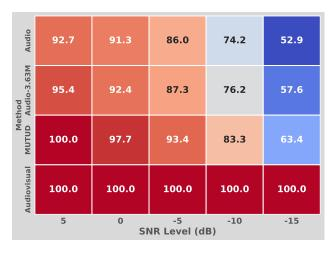
Figure 2: MUTUD bridges the gap between Audiovisual and Audio-only models. Performance (in %) of gain in STOI through different methods relative to the gain *Audiovisual* brings in average intelligibility (STOI) of noisy speech samples. MUTUD is able to get most of performance gains of the *Audiovisual* model across different SNRs. For example, at -5dB SNR *Audio-only* gives gives 86.0% of the gain of the Audioivisual model whereas MUTUD is at 93.4% of Audiovisual model.
