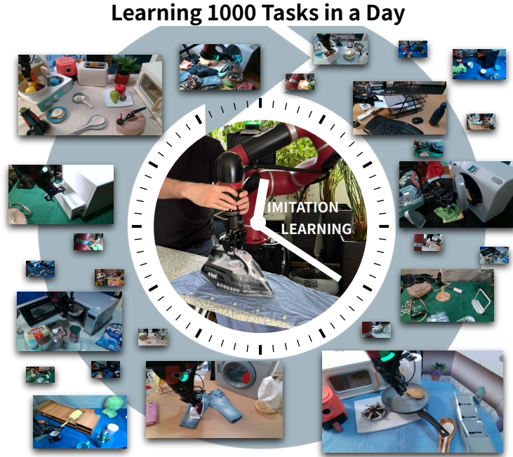
Figure 1: Real-world evaluation rollouts of our MT3 system learning 1,000 tasks from a single demonstration each, all collected in 17 hours. A task is defined as an interaction between the robot and a single object. This data efficiency is achieved by decomposing manipulation trajectories into alignment and interaction phases and using retrieval-based methods for each phase, which in our experiments outperform behavioural cloning alternatives when demonstrations per task are limited.
