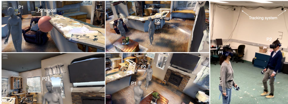
Figure 2: Overview of our data collection system in VR. Sets of two participants took part in the data collection process, wearing a VR headset, trackers, and hand controllers. They performed tasks that required walking in a physical space while reaching goals displayed in the virtual space, which matched the physical space in size. In VR, each participant embodies an avatar that matches their real-world behaviors in real time, to enhance awareness of each other’s presence and movements. The motion tracking system and the VR system record the participants’ trajectories and motions in real time. We use Habitat-matterport 3D dataset (Ramakrishnan et al., 2021) to create the virtual scenes.
