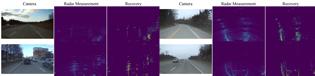
Figure 5: The camera column shows the visual context captured by the camera, depicting the road, vehicles, and surroundings. The radar measurement column displays the low-resolution radar range-azimuth heatmaps y . The recovery column presents the recovered high-resolution angle estimations.
