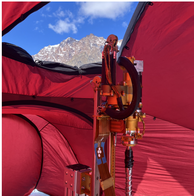
Fig. 1. TRIDENT Drill at Lake Untersee for field testing in Antarctica January 2026
