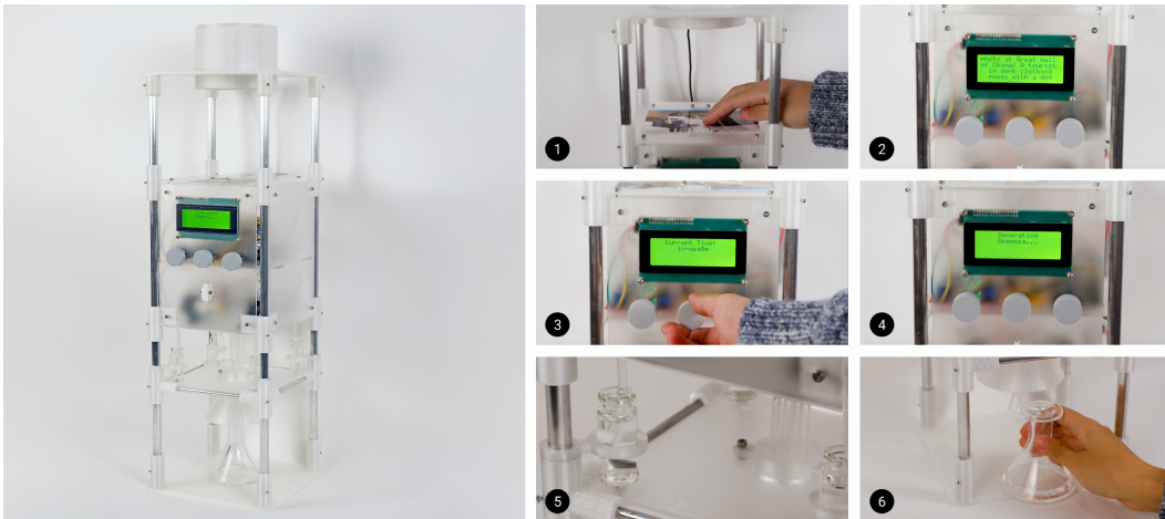
Figure 1: Left: The Anemoia Device. Right: User interaction steps: (1) insert photo, (2) generate caption, (3) prompt via dials, (4) generate story and scent, (5) dispense scent, (6) smell fragrance.
