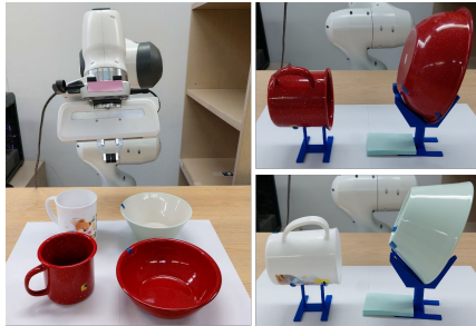
Figure 7: The mugs and bowls used in the real-world experiments along with the Franka Panda robot. The right side of the image shows the mugs and bowls in rotated poses.
