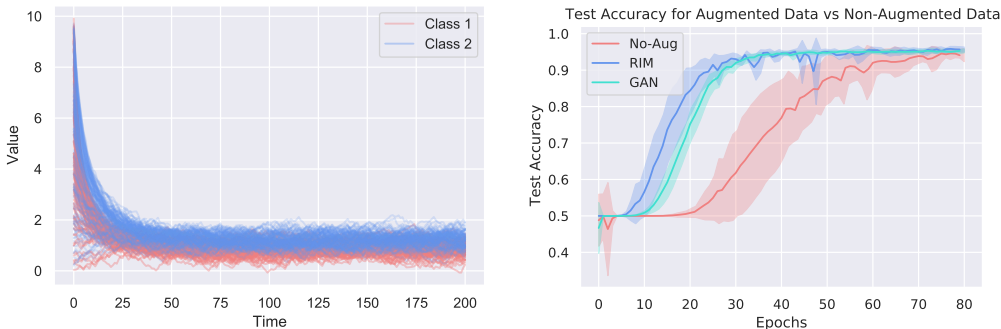
Figure 2: Time series from two classes on the left plot, Test Accuracy for the exponential synthetic ODE system using a Convolutional Neural Network with kernel size=3, filter=32, batch size=16, using BatchNorm and Adam optimizer. The test accuracy plot indicates the resulting mean \pm standard deviation from 10 runs.
