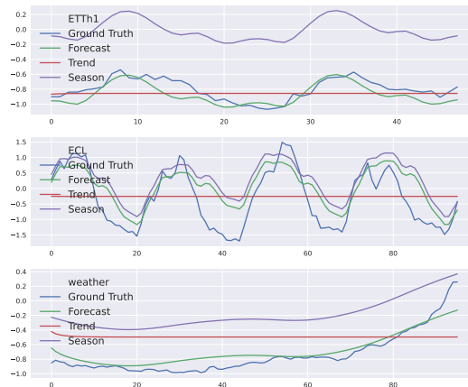
Figure 7: Visualization of decomposed forecasts from ETSformer on real world datasets, ETTh1, ECL, and Weather. Note that season is zero-centered, and trend successfully tracks the level of the time-series. Due to the long sequence forecasting setting and with a damping, the growth component is not visually obvious, but notice for the Weather dataset, the trend pattern is has a strong downward slope initially (near time step 0), and is quickly damped.
