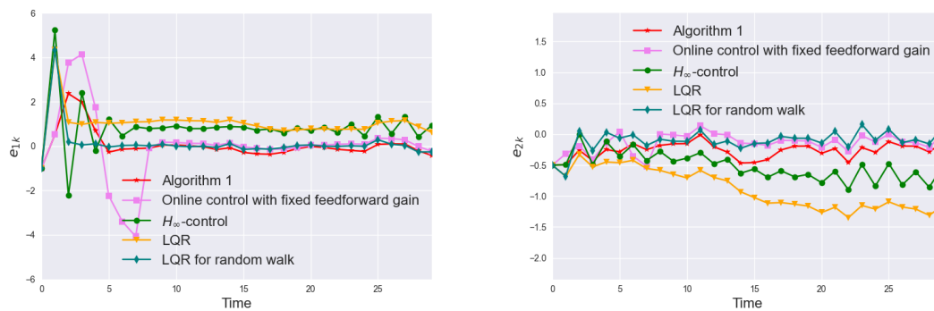
Figure 4: Tracking error for the random walk disturbance for the presented Algorithm 1, versus the online control algorithm with a fixed feedforward gain, the H_\infty control, the LQR control, and the LQR for random walk using the reference signals in Fig. 2.
