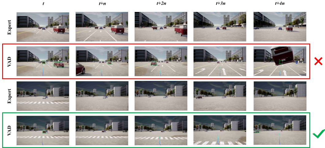
Figure 16: Successful and Failed Cases Behaved in the STR Scenarios: In the failed case, the ego vehicle controlled by the trained VAD model accelerated too slowly while traveling straight, leading to a collision with a trailing vehicle. In contrast, the successful case demonstrated the VAD-controlled ego vehicle navigating the intersection smoothly at an appropriate speed, avoiding any collisions.
