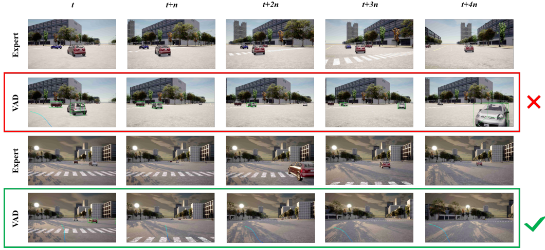
Figure 15: Successful and Failed Cases Behaved in the LFT Scenarios: In the failed case, the VAD-controlled ego vehicle was overly cautious during a left turn and failed to anticipate oncoming traffic, leading to a collision. In contrast, the successful case demonstrated a smooth and well-timed turn, avoiding any interference from oncoming vehicles.
