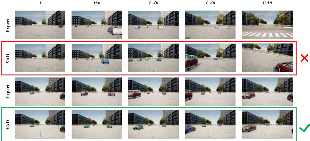
Figure 14: Successful and Failed Cases Behaved in the COV Scenario: In the failed case, the ego vehicle controlled by the trained VAD model exhibited excessive caution while competing for the lane with another vehicle, failing to account for a car approaching from the right rear. This oversight led to a collision due to the ego vehicle’s slow speed. Conversely, the successful case demonstrated effective lane competition at a reasonable speed, avoiding any collisions.
