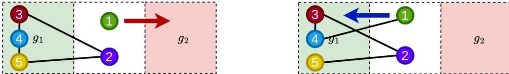
Figure 8: A visual example showing the importance of keeping the CG connected. (Left) CASEC disconnects agent 1 from the rest of the group, failing to obtain the optimal solution. (Right) \xi -sparsification employed by KINGS ensures that the group stays connected and arrives at g_1 .
