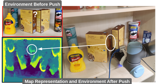
Fig. 1: Motivation of our approach. The robot aims to create a complete 2.5D occupancy height map of the shelf board, which is challenging due to large objects blocking the view. However, by manipulating the right box, the information value of the viewpoint increases significantly due to the newly uncovered object (white circle).
