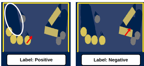
Fig. 4: Two object configurations with a sampled push candidate for each (red arrow). Brighter colors indicate higher object height. Unknown space is marked in dark blue. Labels indicate expert evaluation of push candidate quality in terms of invasiveness and additional uncovered space.
