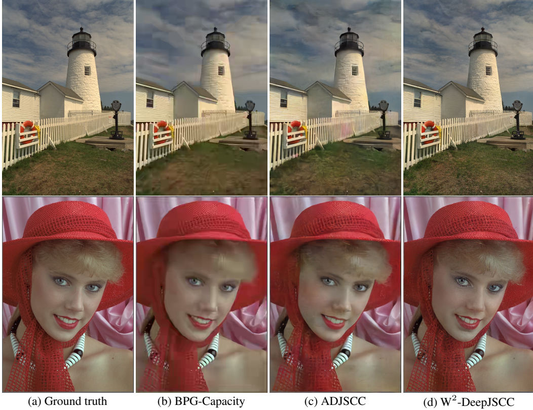
Figure 7: Visual comparisons at SNR = 0 dB and R = 1/24 , where our method demonstrates clear advantages across the entire image. Additional examples are available in Appendix D.
