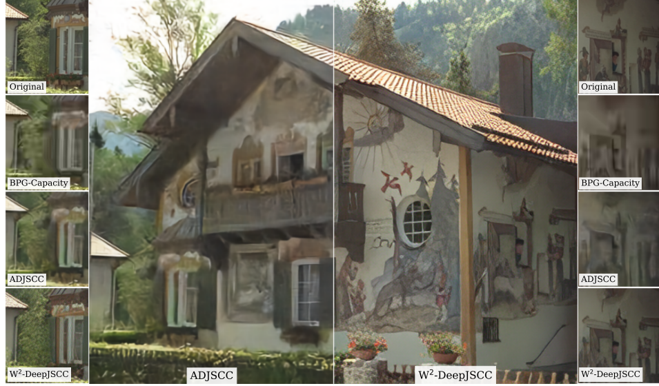
Figure 1: Visual comparison between our W^2 -DeepJSCC, ADJSCC, and the BPG-Capacity scheme when SNR=0dB and R=1/24 . W^2 -DeepJSCC achieves best perceptual realism, closely matching the original image, while others lose significant texture detail. Many more results, including a prototype validation, across SNRs and datasets are available in Appendix and the supplementary materials.
