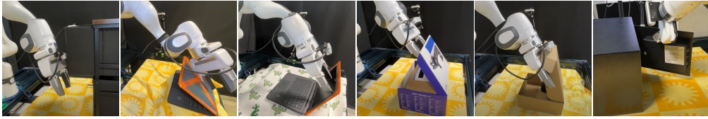
Figure 7. Real Experiments: We observe that the multi-task policy, trained on simulation data, can perform robustly on various unseen real-world objects through sim-to-real transfer.
