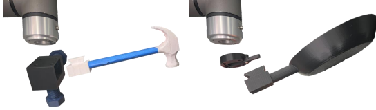
Fig. 6: Fast Tool Changer. Two designs are shown: the left accommodates general tools with a screw mechanism, and the right clips onto tools with specific mounting shapes.
