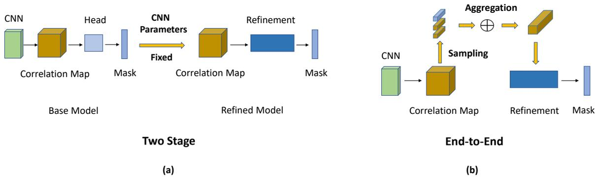
Figure 1: (a): Two-stage SiamMask; (b): End-to-end E3SN. The proposed sampling strategy alleviates the training gap of SiamMask.
