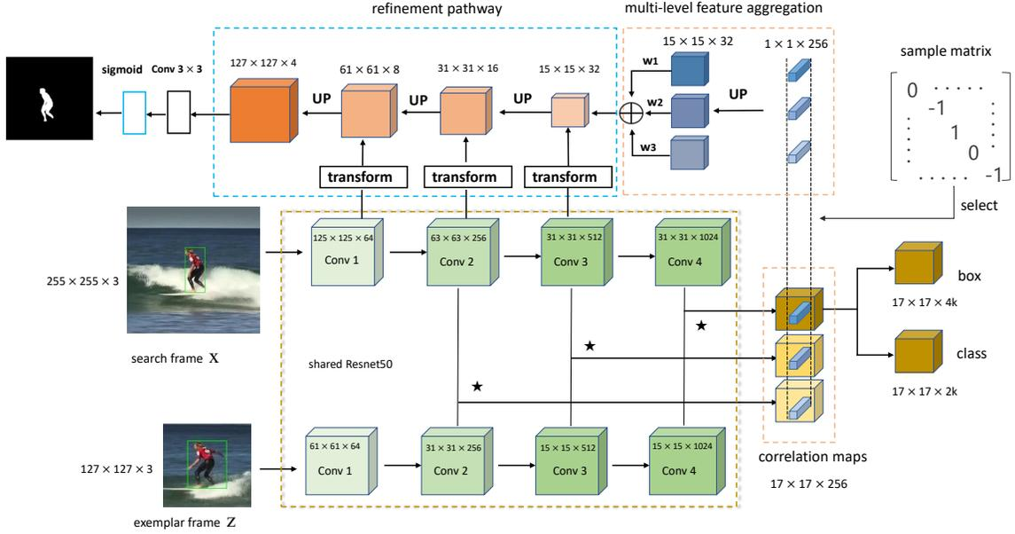
Figure 2: Architecture of the proposed E3SN. Multiple correlation maps are calculated on the basis of multilevel features extracted by the shared Siamese network. A fixed number of positive and negative samples are selected from the correlation maps, and these samples are aggregated for the final mask refinement module.
