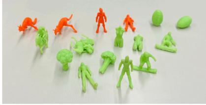
Figure 2: 3D-printed figurines created with Atlas3D stand stably, while those without Atlas3D have fallen down.
