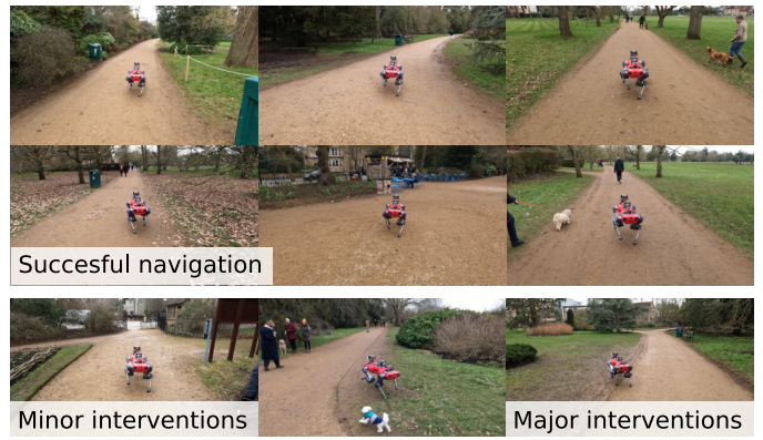
Fig. 4: Kilometer-scale navigation: We deployed our system to learn to segment the footpath of a park after training for a few steps. We executed 3 runs starting from different points in the park: run 1 (0.55 km), run 2 (0.5 km), and run 3 (1.4 km). Minor interventions were applied to guide the robot in intersections; major interventions ( \star ) were required for some areas when the robot miss-classified muddy patches for the path.
