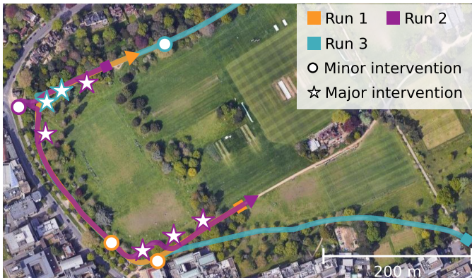
Fig. 4: Kilometer-scale navigation: We deployed our system to learn to segment the footpath of a park after training for a few steps. We executed 3 runs starting from different points in the park: run 1 (0.55 km), run 2 (0.5 km), and run 3 (1.4 km). Minor interventions were applied to guide the robot in intersections; major interventions ( \star ) were required for some areas when the robot miss-classified muddy patches for the path.
