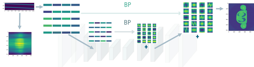
Figure 2: RecoNet with multi-scale backprojection operators. Five skip connections incorporate backprojection operators with varying geometrical resolutions: the original full-resolution and four progressively downsampled (factors of 2, 4, 8, and 16).
