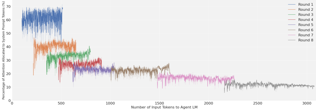
Figure 4: The phenomenon of attention decay demonstrated in the 11th attention head in the 24th layer of LLaMA2-7B, which has a maximum context window size of 4,096 tokens. We generate 12 conversations while tracking the portion of attention allocated to system prompt tokens. The plots are specifically for the agent LM, grouped by the rounds in which the answers are generated; the values are absent for the user LM. We observe sharp drops in attention between turns and rough plateaus within turns.
