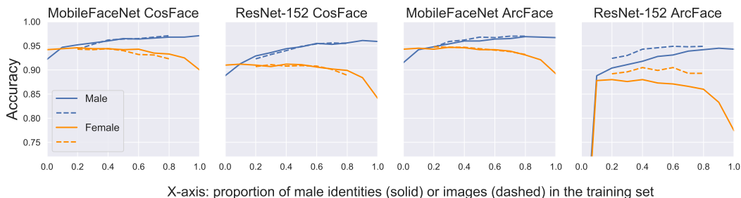
Figure 8: Train Set Imbalance Results of experiments that change the train set gender presentation balance for models trained without class-balanced sampling . Male (blue) and female (orange) accuracy are plotted against the proportion of male data in the train set. All models are tested on the default balanced test set.
