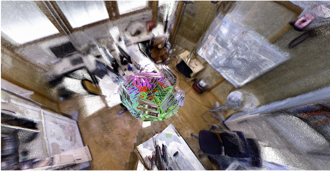
Figure 12: Visualization of reconstruction on TUM 360 scene with 6 submaps. Camera pose estimates are colored by submap. Part of the scene is cropped for visual clarity.
