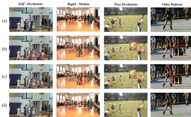
Figure 4: The keyframe (a) and visual comparisons of detection results obtained from DCPose (b), TDMI (c), and our JM-Pose (d) on challenging scenes in the PoseTrack dataset. Inaccurate predictions are highlighted with the red solid circles.
