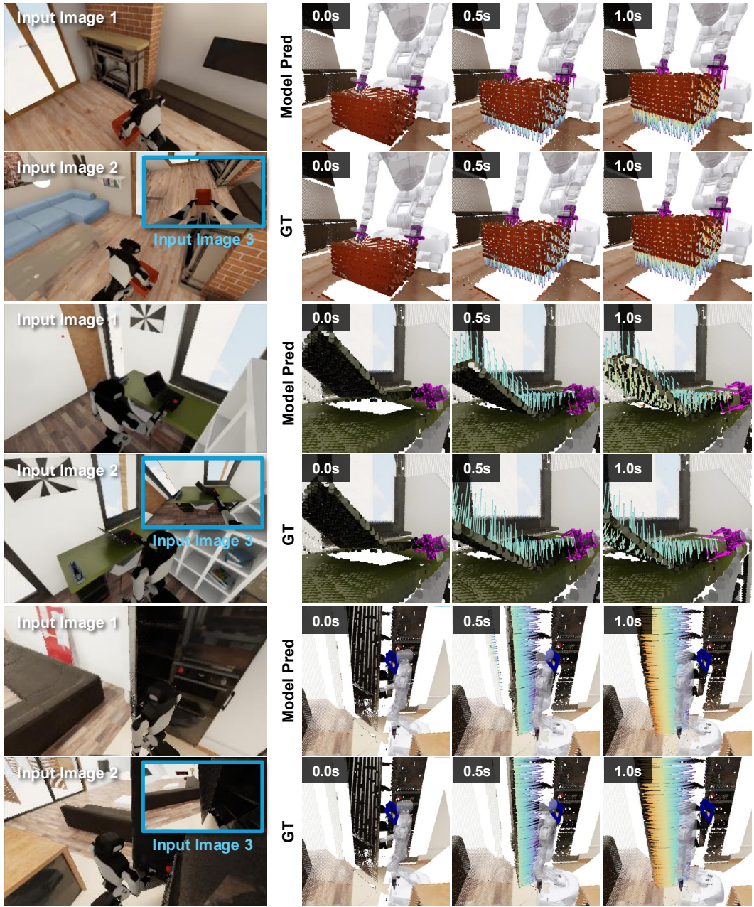
Figure 19: BEHAVIOR-1K Unseen Rollouts , including constrained bimanual lifting, gravity effects (dropped laptop), object-object interactions (laptop v.s. table), and articulated manipulation (fridge).
