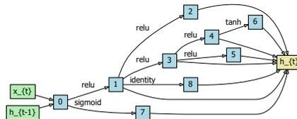
Figure 3: The recurrent cell searched by our approach on the Penn Treebank dataset. The random seed is 3.
