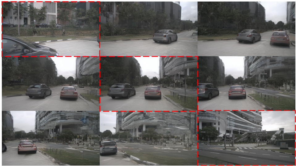
Figure 14: Visualization results for inserting 3 virtual cameras on both sides of the front camera with different yaw angle. 3 views with red border are front-left camera, front camera and front-right camera of nuScenes dataset, while others are virtual cameras.
